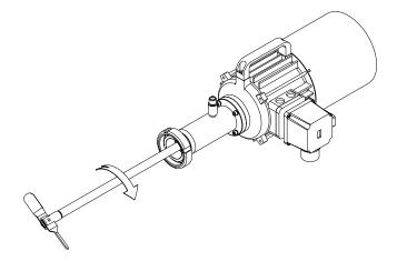
Start up the agitator motor briefly. Ensure that the direction is consistent with the one indicated on the plate. If the agitator operates in the wrong direction, the folding propeller may fall into the tank.
